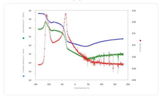
A DMA curve from -150 °C to 180 °C at 3 °C/min is shown. A glass transition is observed at -107 °C, and a crystalline melting transition is observed at -37 °C followed by a rubbery plateau to the conclusion of the test at 180 °C.
